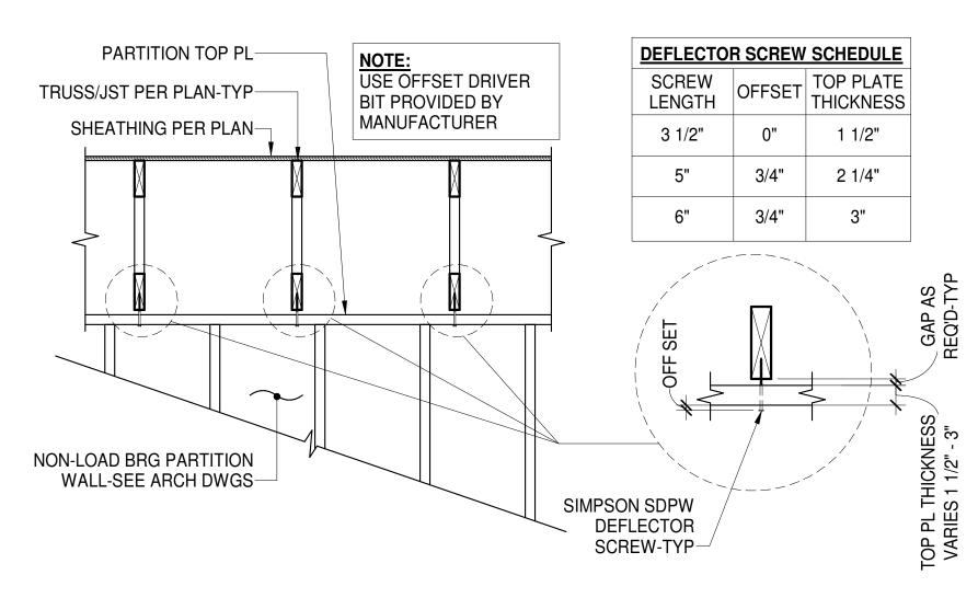
F TYP SLIP CONNECTION @ NON LOAD-BRG WOOD PARTITION WALL ൃ S1.5 ⊱ N.T.S.
