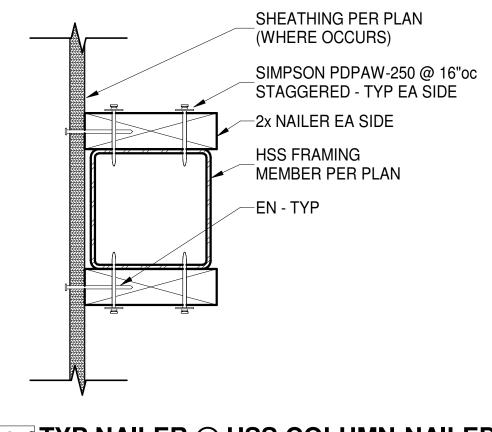
TYP NAILER @ HSS COLUMN-NAILED | S1.5 | N.T.S.
