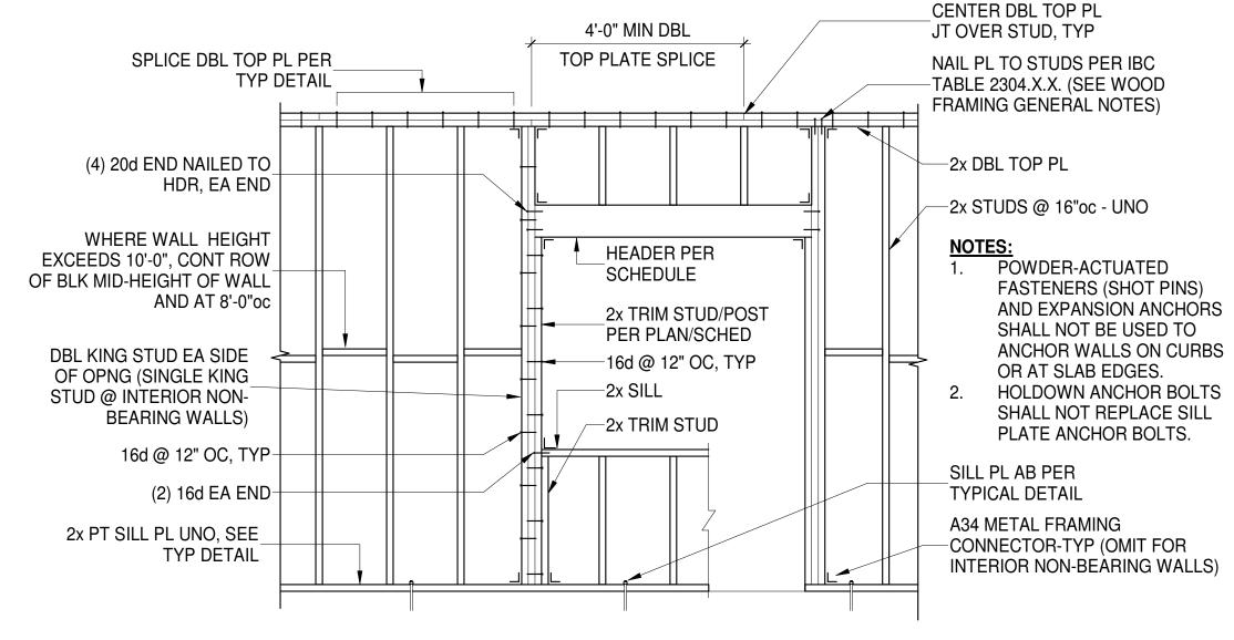
B TYP STRUCTURAL WALL PANEL FRAMING ELEVATION
