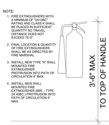
A5 TYPICAL FIRE EXTINGUISHER DETAIL
