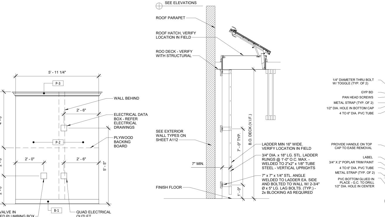
© SECTION AT ROOF LADDER, TYP. N.T.S.
