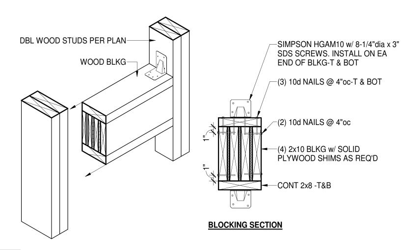
TYPICAL CANOPY ATTACHMENT BLOCKING @ WOOD STUDS N.T.S.
