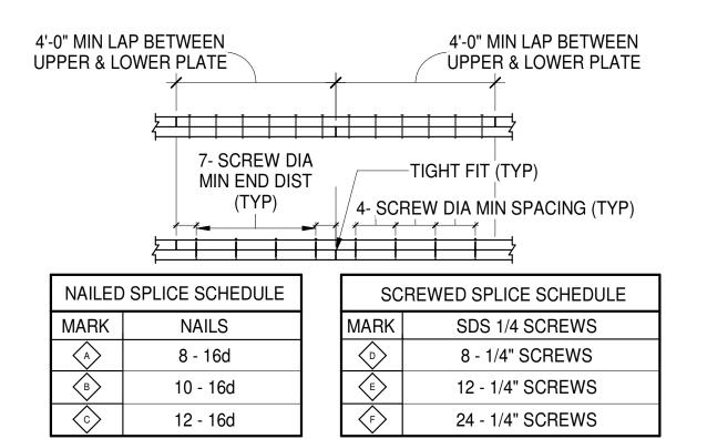
SPLICE 2x DOUBLE TOP PLATES PER MARK "A" AND 3x DOUBLE TOP PLATES PER MARK "D" OF THE ABOVE SCHEDULE, UNLESS OTHERWISE INDICATED.
