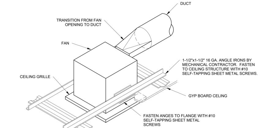
1 CEILING EXHAUST FAN DETAIL NOT TO SCALE
