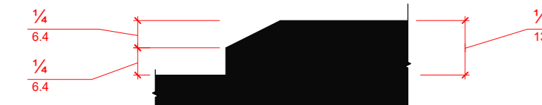
FIGURE 303.3 BEVELED CHANGE IN LEVEL
